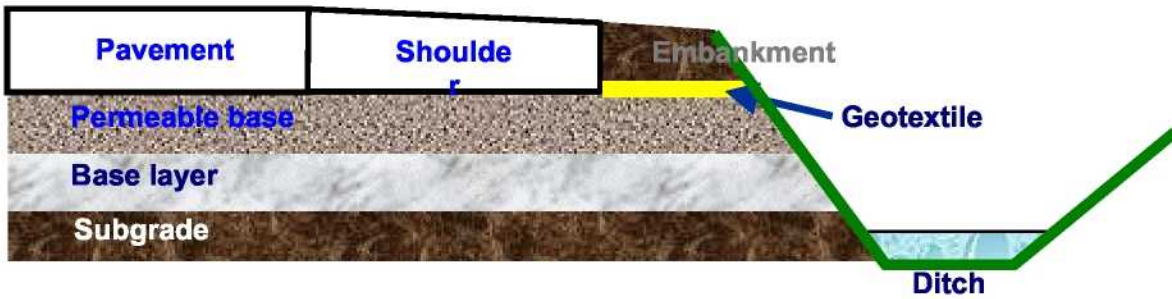
Figure 7-3. Typical AC pavement with a daylighted base.
